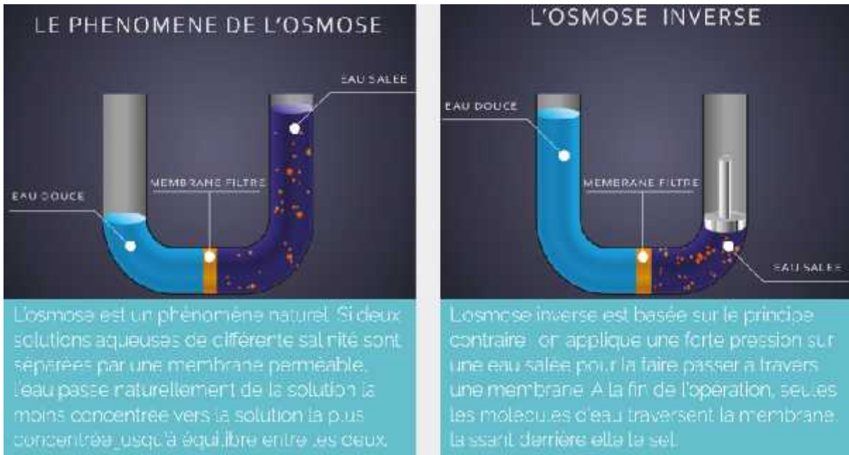
Figure III.4: La technique de désalinisation
