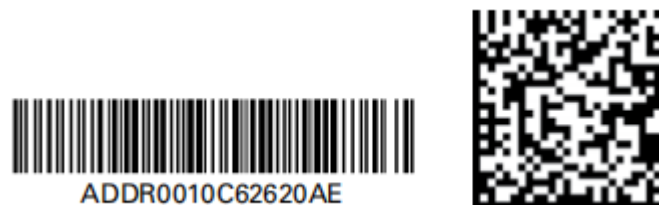
Figure n°1.4: One-dimensional and two-dimensional barcodes
